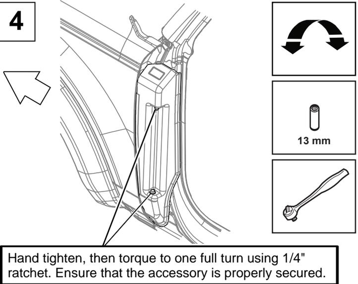
Hand tighten, then torque to one full turn using 1/4" ratchet. Ensure that the accessory is properly secured.
