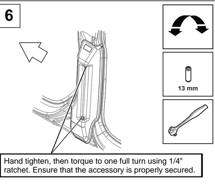
Hand tighten, then torque to one full turn using 1/4" ratchet. Ensure that the accessory is properly secured.
